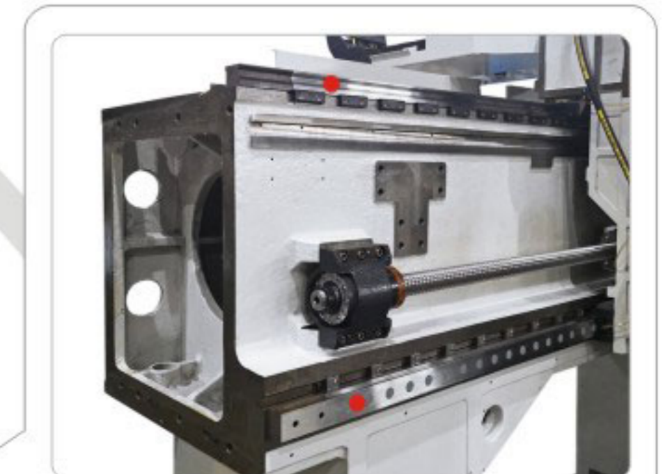
Vertical guideway layout for Y axis
