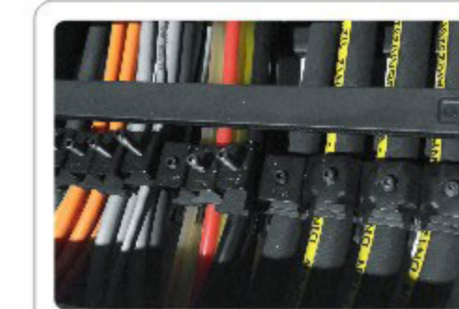
Tank chain cable tubing All cable tubing inside the tank chain uses special made fixtures to avoid cable tangle and rubbing damage.
